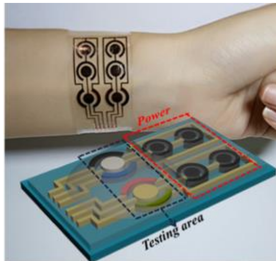
Figure 3. Example of a wearable sensor powered by smart flexible batteries
