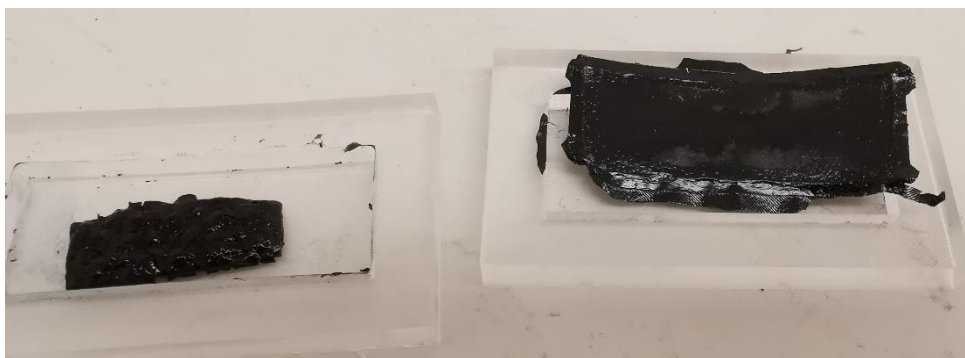
Figure 37. Difference between thick film with salt (left) and without salt (right)
