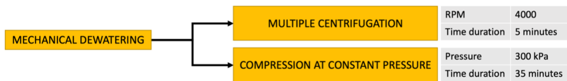
Figure 16 Procedure of mechanical dewatering.
