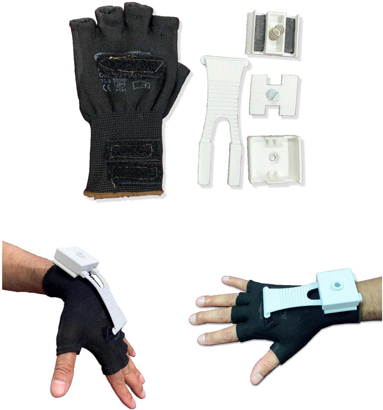
Figure 47: The 3d printed prototype parts and the assembled glove worn and two hand positions are shown.
