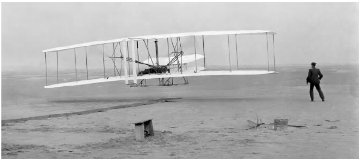
Figure 3: Wright brother's aircraft design used compliant wing warping to ensure a sustained flight for humans
