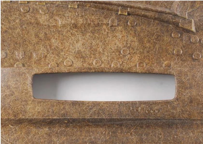
Fig. 20: composito rinforzato con fibre di canapa. Fonte: [www.hashmuseum.com/nl/de-plant/industrial-hemp/hemp-based-plastic](http://www.hashmuseum.com/nl/de-plant/industrial-hemp/hemp-based-plastic)
