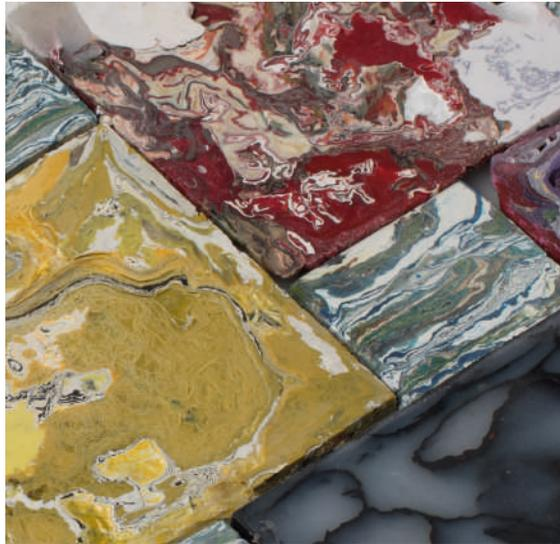
Fig. 34: Plastic Stone Tiles. Fonte: [www.materialdistrict.com/material/plastic-stone-tiles/](http://www.materialdistrict.com/material/plastic-stone-tiles/)
