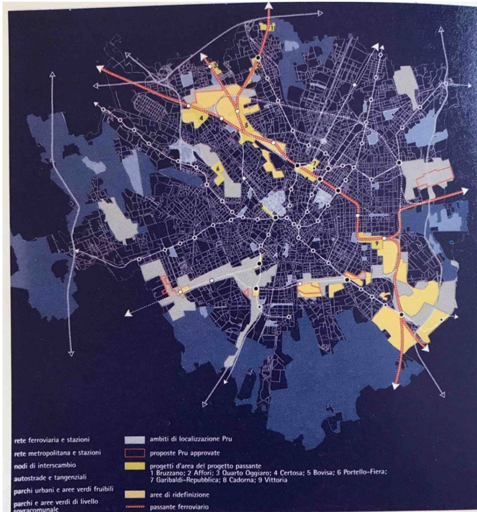
Fig 21. Passante Ferroviario (mainline rail link), area and redefinition projects marked in yellow, zones for the location of PRUs (urban enhancement programs) in grey
