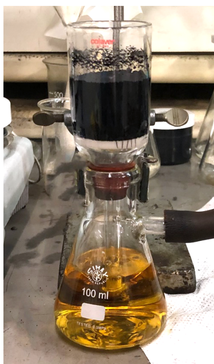
Figure 3.4 - Picture of the filtrate at the end of the first functionalization step. CA: Graphite.
