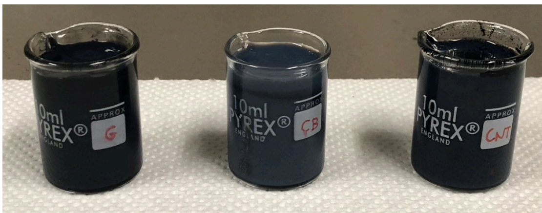
Figure 4.1 – CA-SP-Ag inks prepared dispersing powders in a blend of polycarbonate resin and propylene glycol. From left to the right: G-Ag ink, CB-Ag ink and CNT-Ag ink.
