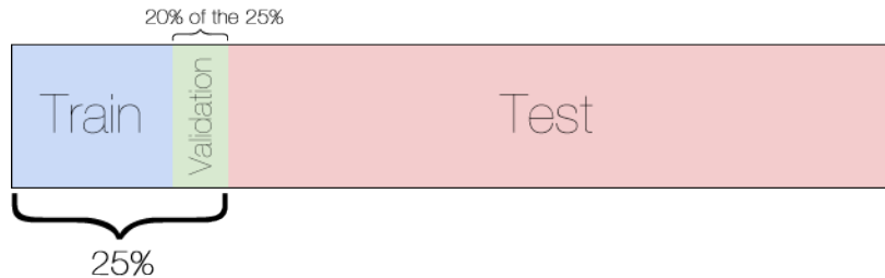
Figure 6.7 In this figure, as an example, we see how we perform the selection of the subset: first, we sample 25% of the target dataset, according to a given criterion - e.g. top 25% for entropy, bottom 25% for entropy, random 25%. Then, we furtherly split the subset to get a validation set.
