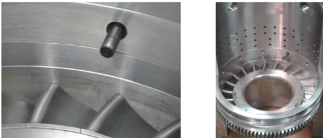
Figure 1.3: Internal view of channel with an EWG injector upstream of the stator
