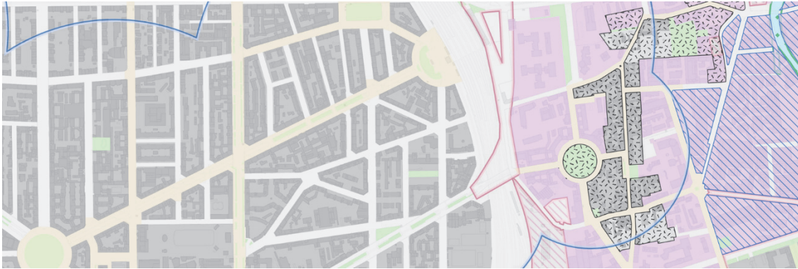
Figure 17. Extract of the plan “R02 Indicazioni Urbanistiche” (planning indications) from the Piano delle Regole (rule plan) of the Piano di Governo del Territorio in force of the Municipality of Milan. The blue line incorporates “areas with high accessibility to public transport network”. Source: MILANO 2030 - Piano di Governo del Territorio (2019), Comune di Milano
