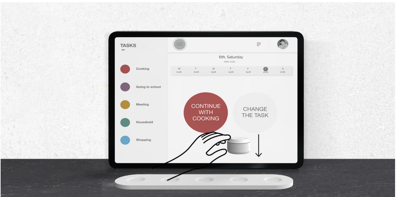
14. If she needs to add more tasks in her system, she put the NADI in the first place of the interactive base. Or, if she wants to change the task that has already saved in the system after confirming, she again puts the NADI on the place that she wants to change. And, the system asks whether she wants to change the task or add a new one.
