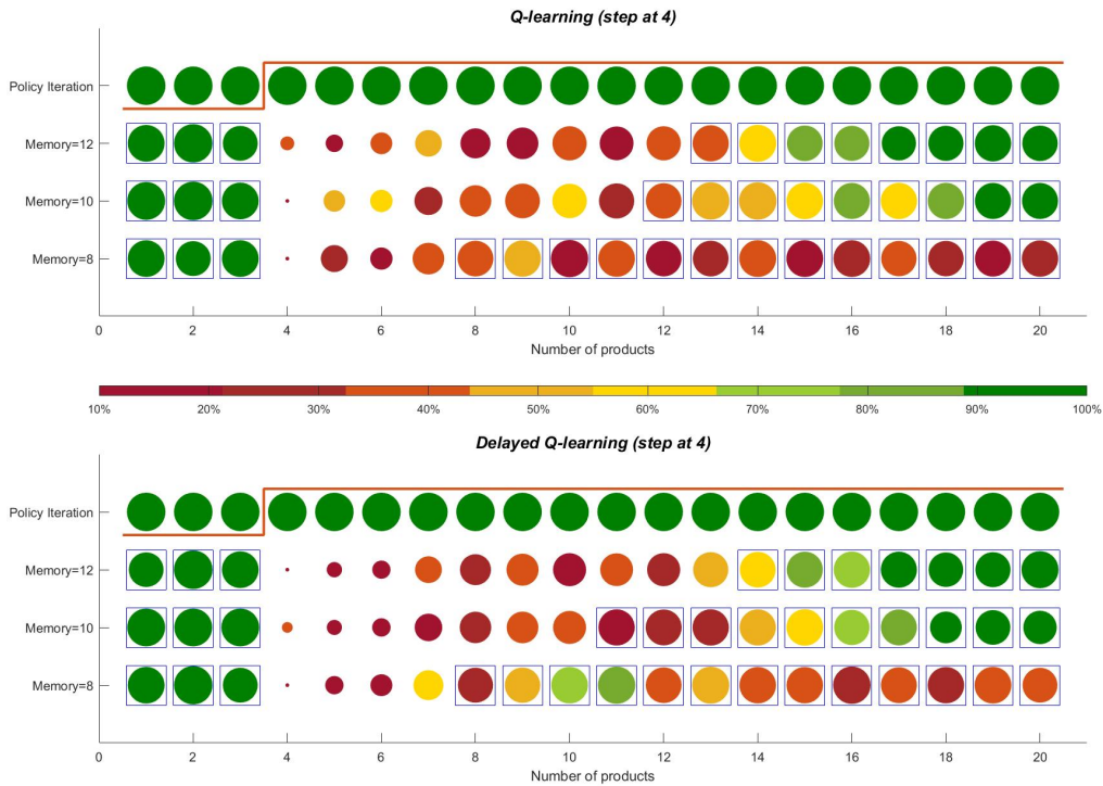
Figure 7.2: Plot of the performances with Q-Learning (top) and Delayed Q-Leaning (bottom). Each circle represents a optimal scheduling returned by a technique. The circle size measures the closeness of the optimal scheduling cycle time to the reference one (larger implies closer). The circle colour measures the probability that the optimal scheduling is the reference one (green implies high probability)
