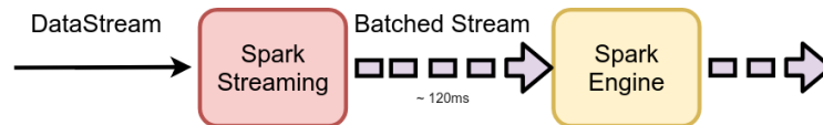
Figure 2.5: SparkStreaming library collects continuous inputs streams in data batches every 120ms before processing
