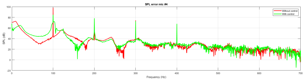
Figure 4.22: Noise spectra at error microphones 3 and 4
