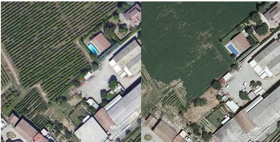
Figure 5.21: Quality comparison between Mapbox (left) and Orthophoto (right) sources. In these images there are also two squared polygons containing wastes, collocated in the same geographical position in both the images.
