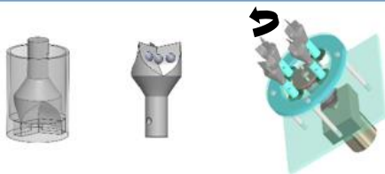
Figure 2 The protocol involves dip-coating, calcification embedding and polymerization in ad-hoc designed Spinning Device.
