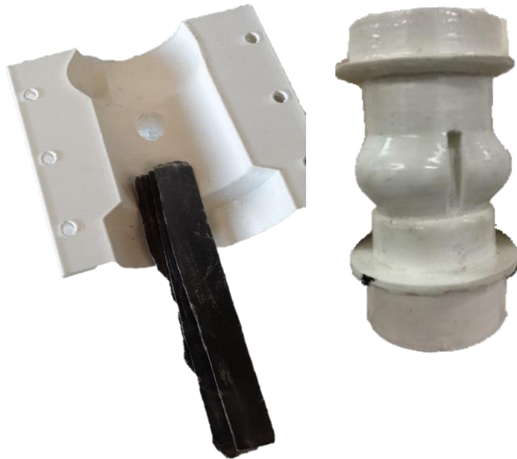
Figure 67 Molds undergoing Post-Processing phase: rubbing down process via sanding paper on the left and brushing XTC-3D coating on the right.
