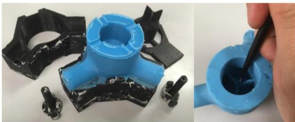
Figure 52 In blue, silicon (GLS-20PRO) casted inside of the PLA-mold, in black. [4]
