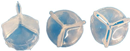
Figure 10 Physiological Aortic Valve Model obtained through dip-spin coating of Sorta Clear 18.
