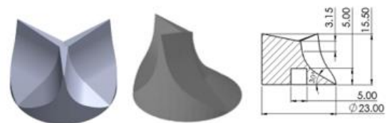
Figure 6 Tricuspid and bicuspid realistic CAD models.
