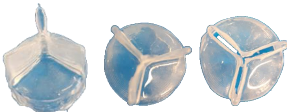
Figure 95 Physiological Aortic Valve Model obtained through dip-spin coating of Sorta Clear 18. Frontal, top views. On the right the free edge is cut through a cutter.
