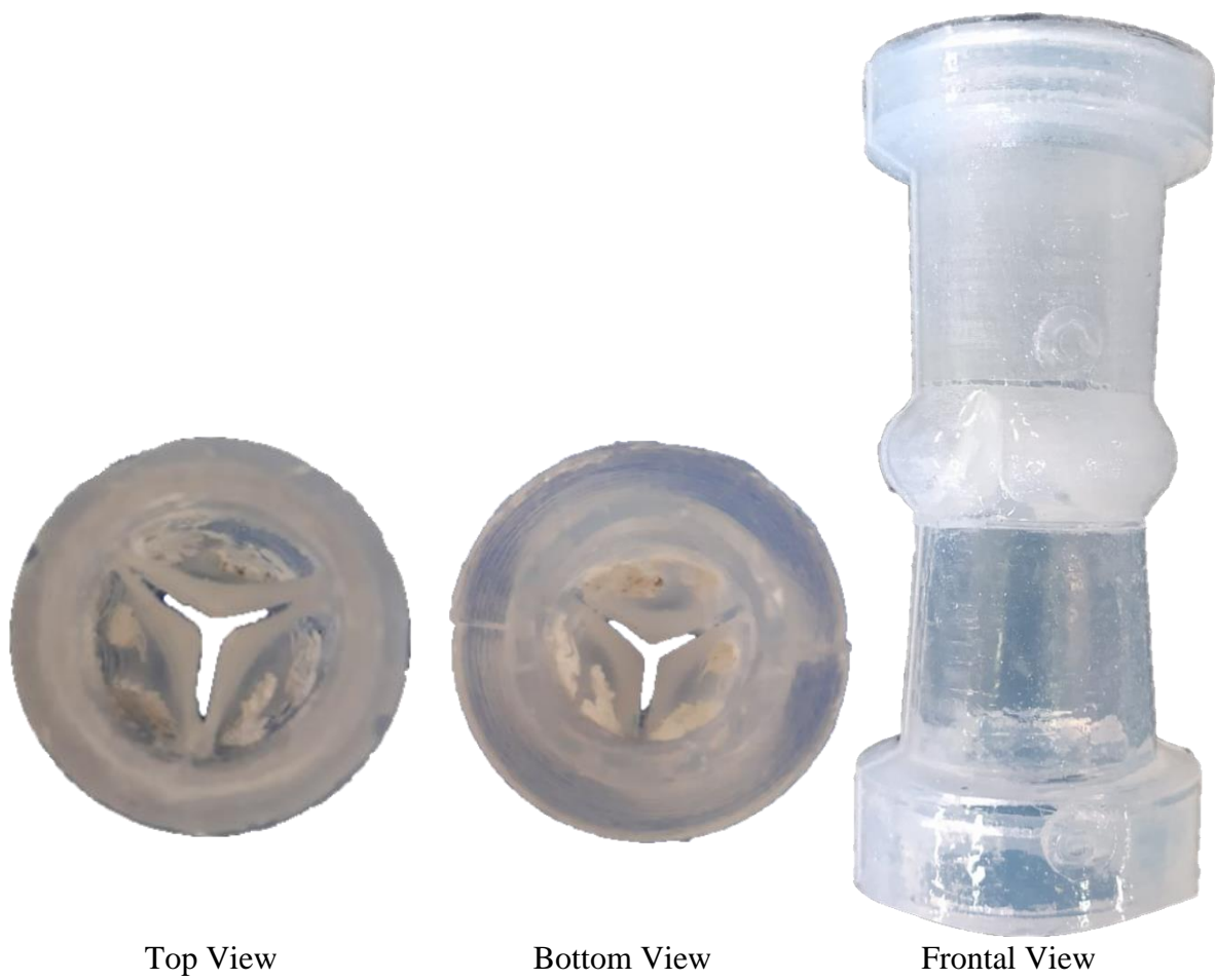
Figure 96 Prototype of preliminary AR model. It includes AV with partial arc calcification pattern.
