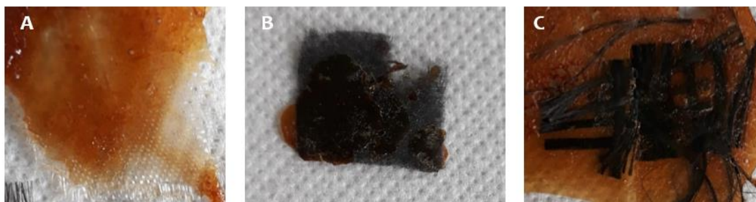
Figure 4. 40 Examples of Composites: A with glass fibers, B with non-woven carbon fibers, C with woven carbon fibers
