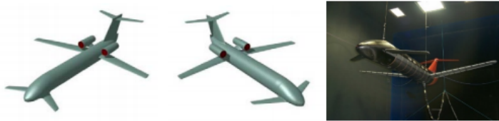
Figure 2.1: Wind tunnel configuration of the old X-DIA model.
