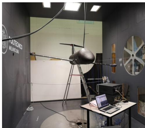
(b) Wind tunnel configuration GVT.
