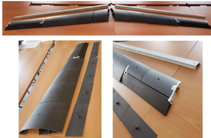
Figure 2.6: Right wing, left wing, ailerons and spars.
