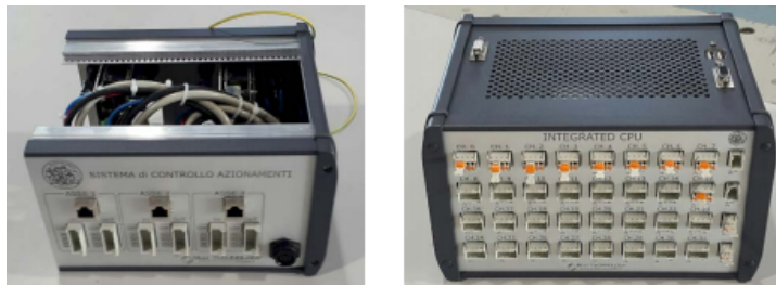
Figure 2.11: Box containing the drive control system (left), built-in computer with data acquisition system (right).
