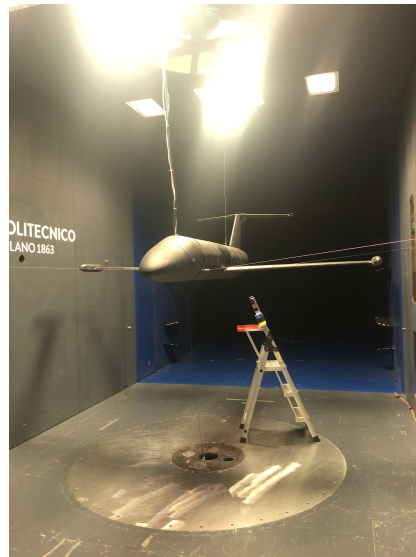
Figure 2.9: Free-free constraint in the wind tunnel.
