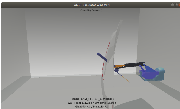
Figure 4.11: Soft body issue: interpenetration between the robot and a cloth. In this case the simulation is too slow and the PSM is not controllable
