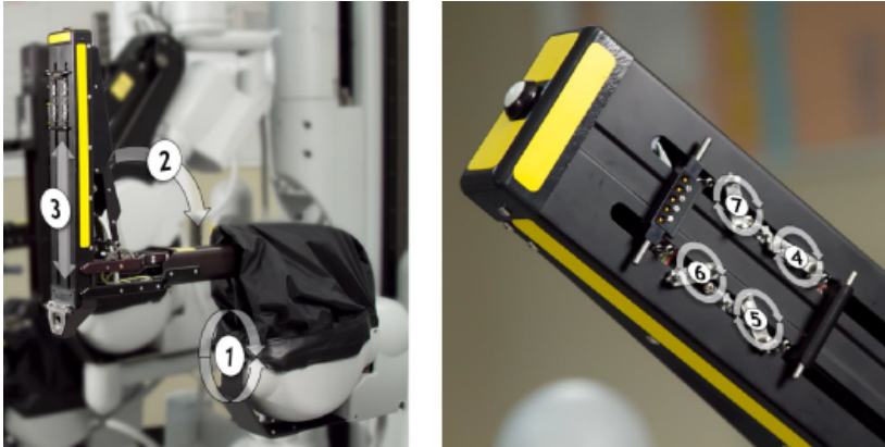
Figure 4.1: The 7 joints of Patient Side Manipulator. Image taken from the dVRK User Guide [49]
