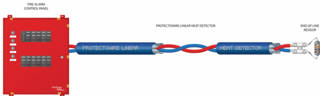
Fig.4-16 Line heat detector (Source: Robert C., Other detection and alarm devices. 2018)
