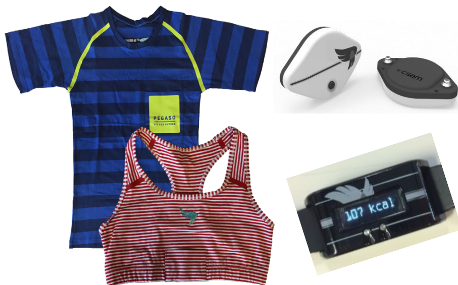
Figure 30 – PEGASO Sensorised garments (initial design); PEGASO Data Logger (connected to the garments); PEGASO Bracelet (showing calories consumption)
