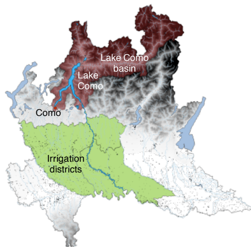
Figure 7.2: Digital Elevation Model of the Lombardy region, Italy. The highlighted elements are Lake Como and its Alpine basin, the sublacual Adda River, the city of Como and the downstream irrigation districts.
