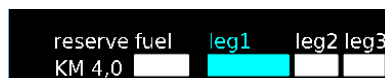
Figure 6.3: Fuel gauge for reserve fuel, and fuel assigned to legs one, two, and three.
