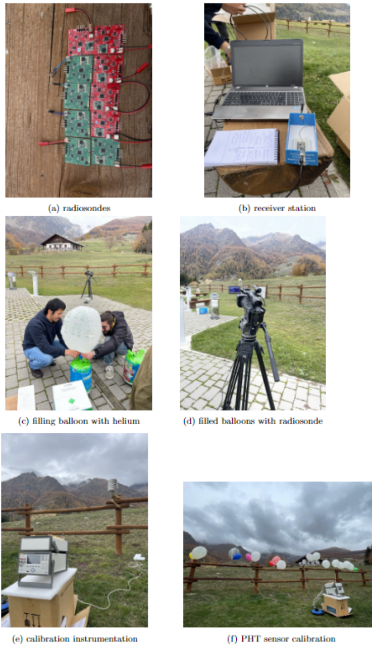
Figure 6.7: Experiment setup with (a) 10 radiosondes, (b) 2 ground stations, (c) 2 cameras, and (e) calibration instrumentation.
