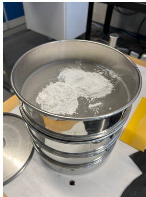
Figure 2.3: Different size 1393B20 glass powder before sieving.
