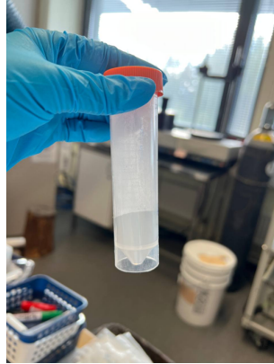
Figure 2.4: 1393B20 Glass powder with size <38\text{ }\mu\text{m} .
