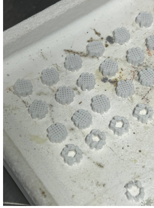
Figure 2.5: Cylindrical and hollow scaffolds before sintering.
