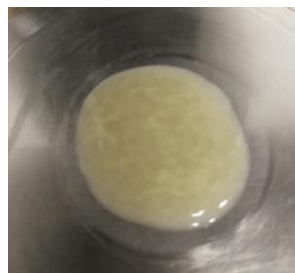
Figure 4.18: macroscopic view of frozen and successively defrosted samples when pipetted on the rheometer plate
