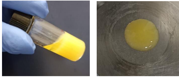
Figure 4.34: macroscopic view of how the mucus model appears after 30 days of storage in the vial and on the rheometer plate before providing the test
