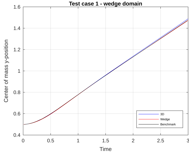
Figure 6.10: Center of mass position evolution. Comparison between uniform grid and wedge case for test 1 (with h = \frac{1}{128} ). Benchmark values from [23].
