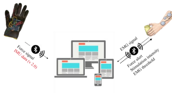
Figure 51: System communication architecture.
