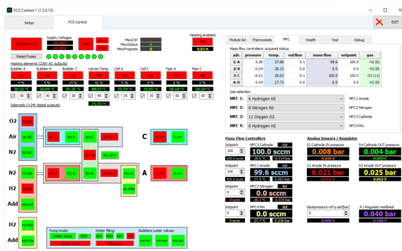
Figure 2.6: Example of the screen of the custom control software.
