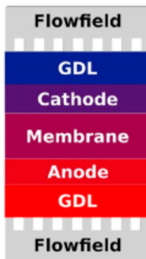
Figure 2.2: Schematic representation of the MEA structure [35].
