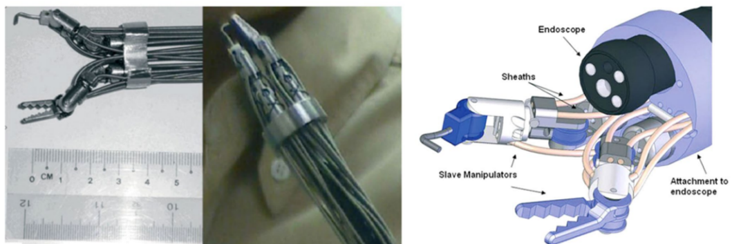
(a) MASTER's the two robotic arms' end effectors (b) system attached to a conventional endoscope
