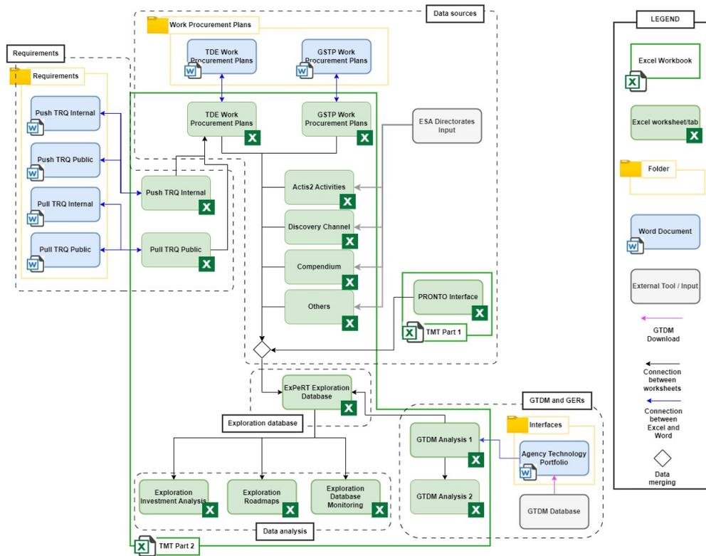
Figure 3.25: TMT Part 2 logical architecture
