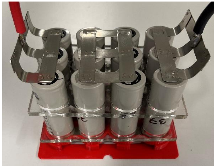
Figure 23 Battery Module Configured in a 3P4S Arrangement(Avik, 2024).
