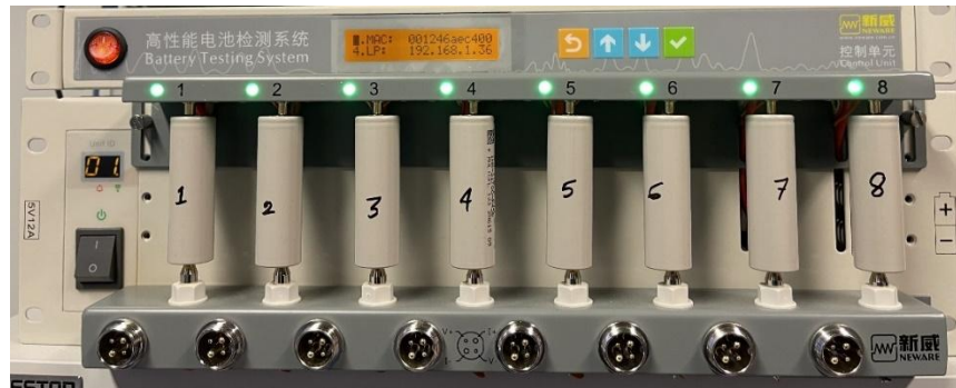
Figure 24 Single-cell testing was conducted using the Neware battery cycler(Avik, 2024).
