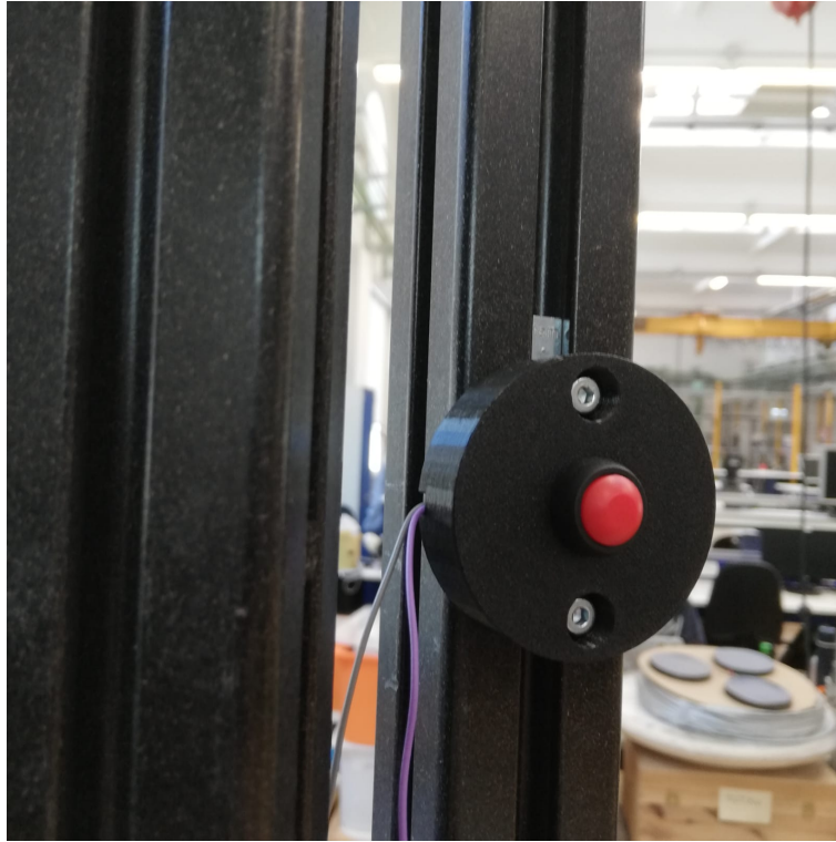
Figure C.8: The "ESC" button within its case. Cables have a small canal in the back to safely get outside without getting smashed
