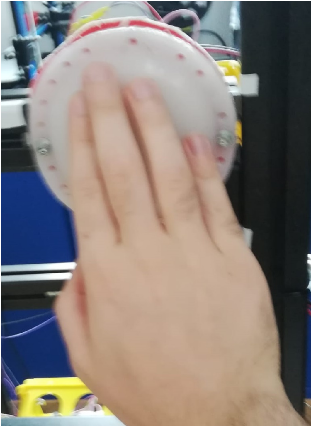
Figure E.1: Here the ideal hand position to trigger the sensors is represented.
