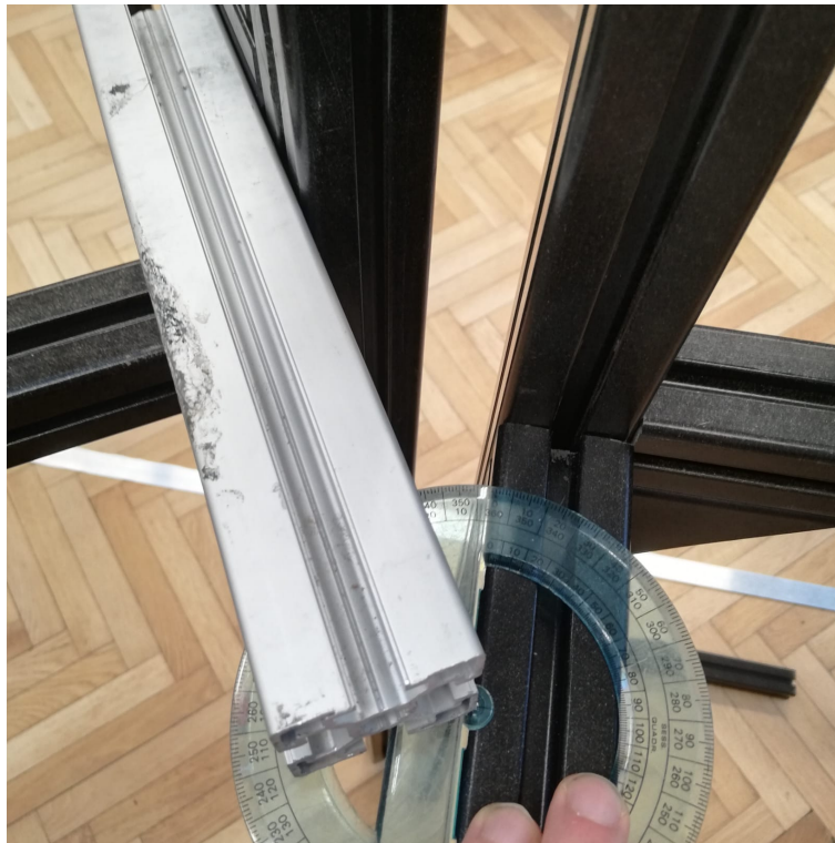
Figure D.3: Image showing one way to use a goniometer to set the aperture angle.
