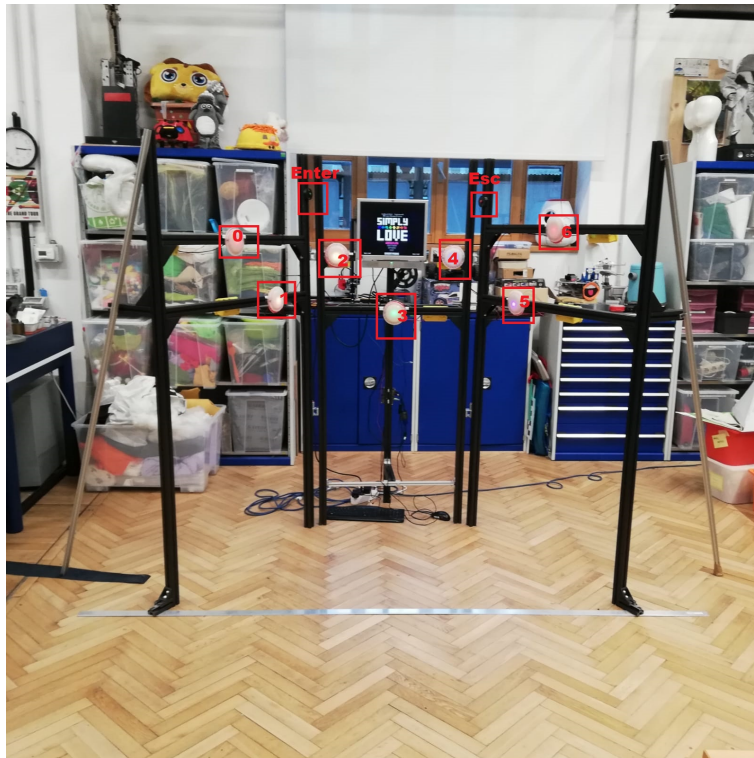
Figure D.1: Image of AIR ExDaMa. Every sensor is here associated with their corresponding ID/key.
