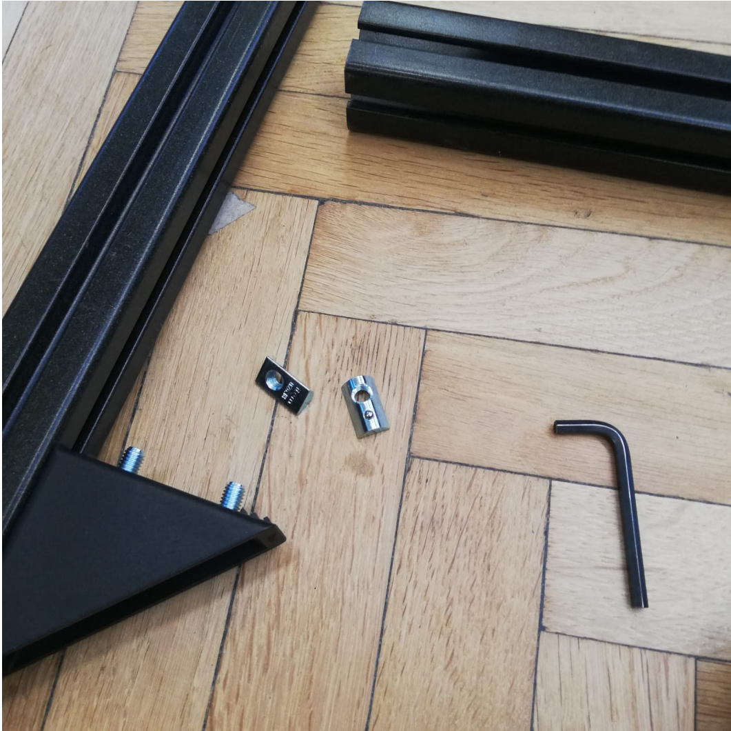
Figure B.4: Image showing a triangular bracket fixed only on one side.
