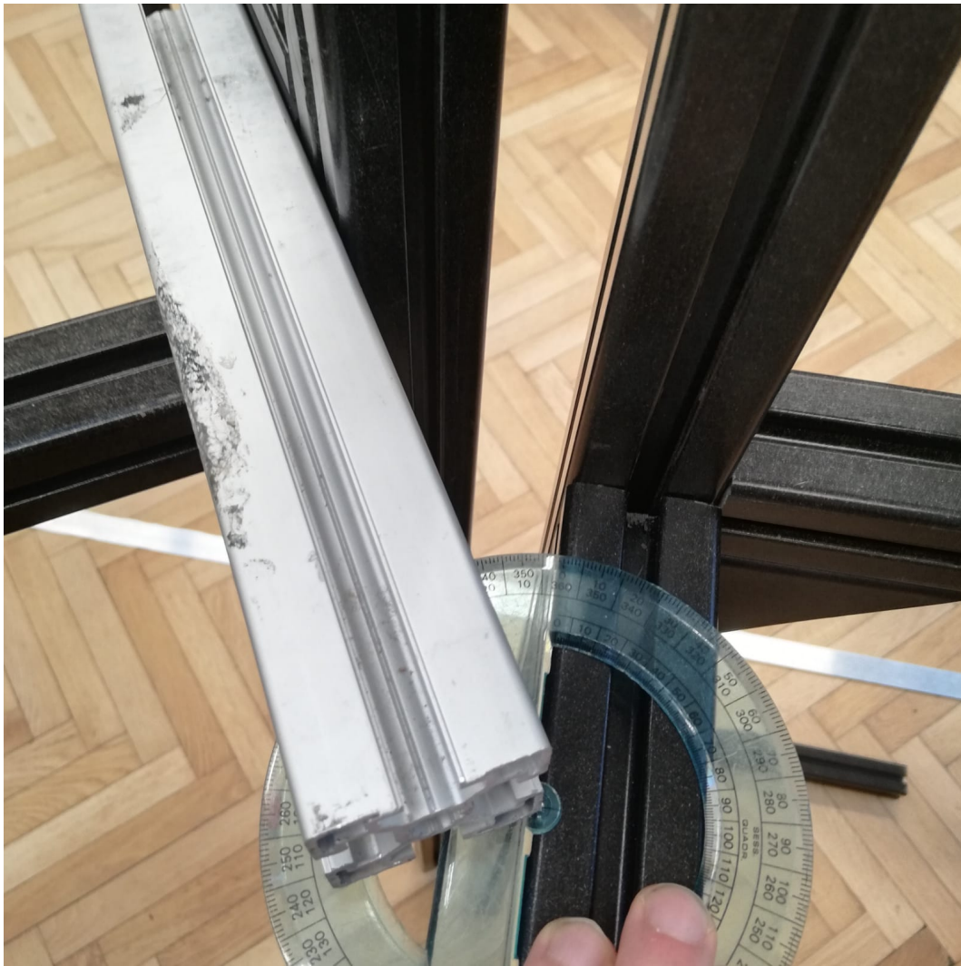
Figure B.5: Showcase of the goniometer use for setting up the aperture angle.
