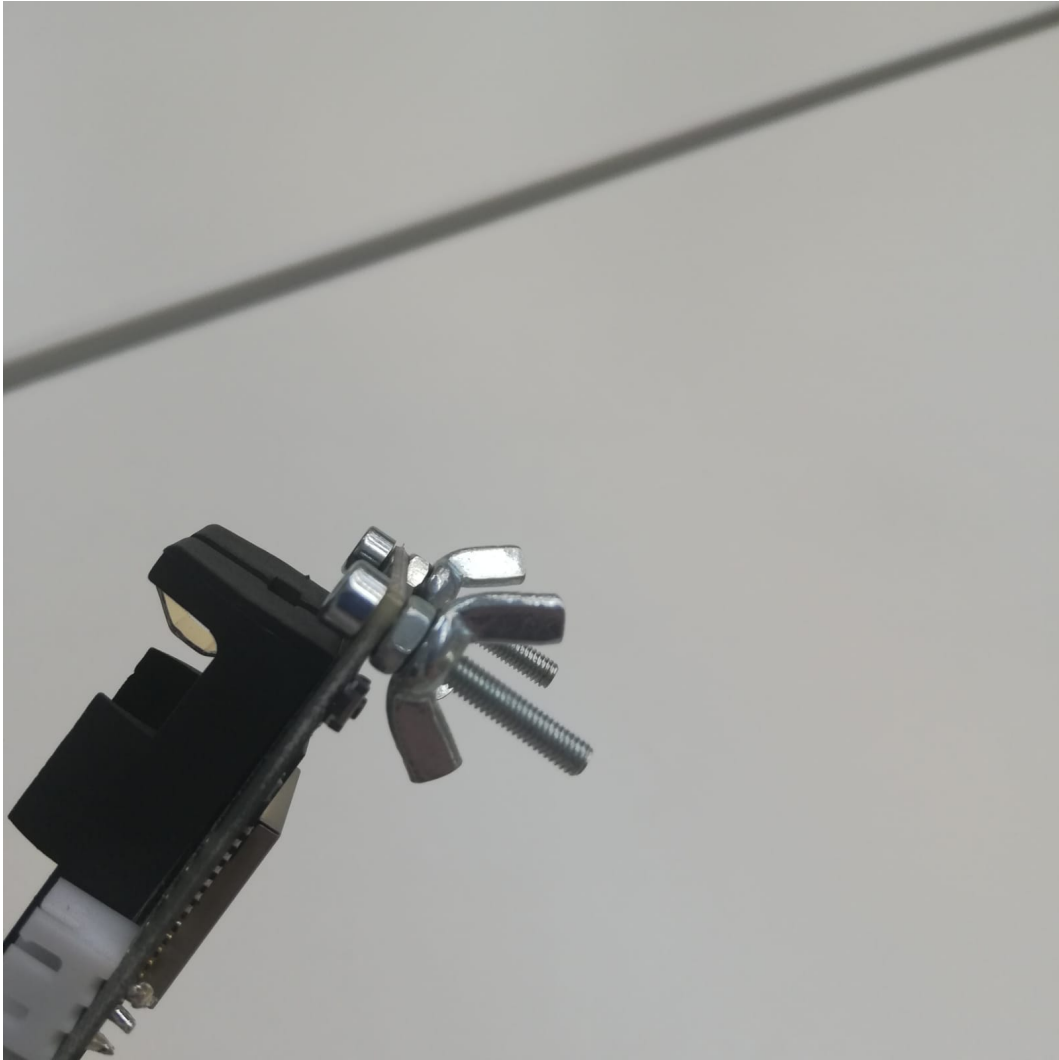
Figure B.9: Image showing how nuts are used to keep the ESPs floating inside their box.
