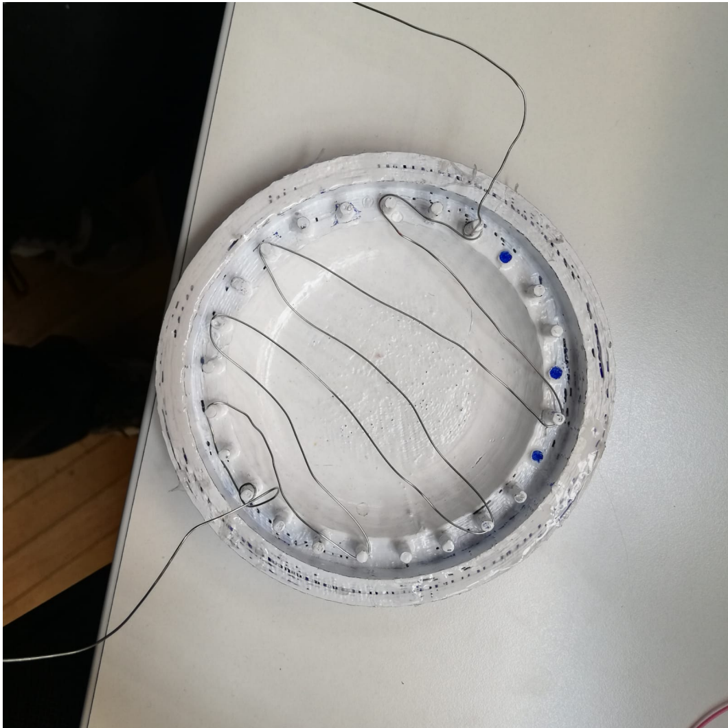
Figure B.8: Image showing the used cable pattern for the produced sensors.
