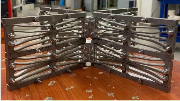
Figure 7 : Picture of the third iteration model in the deformed state after the second dynamic compression test
