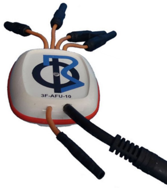
Figure 2.12: Anti-fatigue units - www.3-x-f.com . The single input pin should be connected to the stimulation cable. The stimulation pulses are split to the four electrodes connected to the output pins
