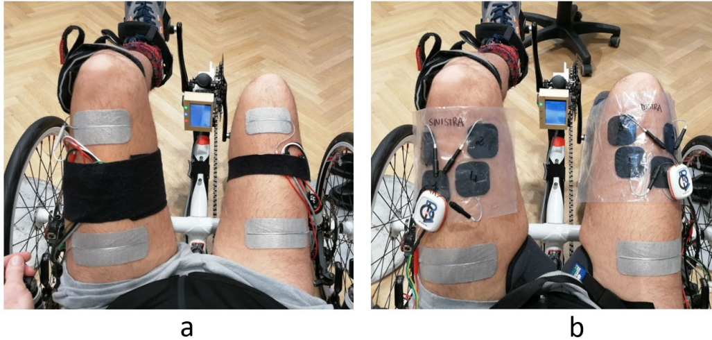
Figure 2.13: a. Electrode placement for testing at constant stimulation (30Hz, 40Hz, DFT) b. Electrode placement for spatially distributed sequential stimulation
