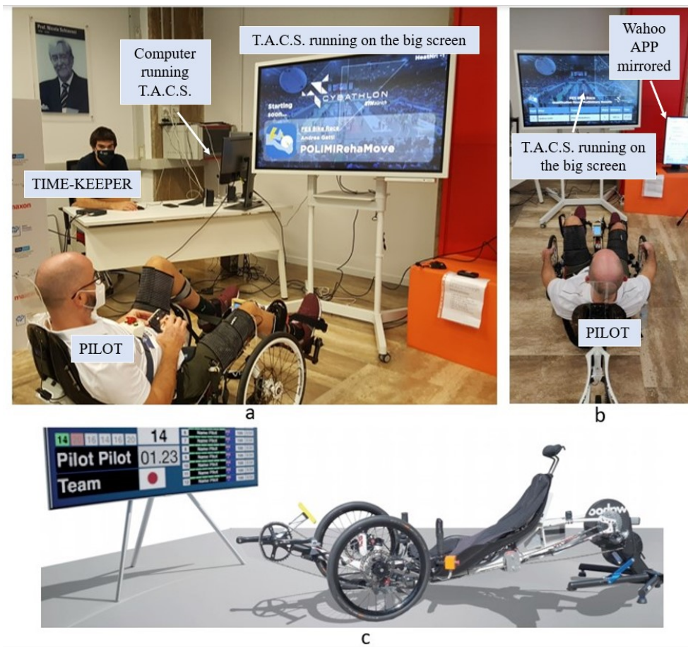
Figure 2.9: a. A picture of the day of the race where it is possible to see the time-keeper on the left side with the computer running T.A.C.S. and the smartphone running the Wahoo app. b. In front of the pilot the big screen is synchronized with T.A.C.S. while the small screen is mirroring the Wahoo app c. Scheme of the set-up provided by the organizers.
