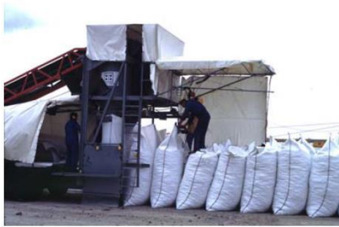
Figure 2.20. Photograph of filling plant for geosynthetic containers ( Heibaum, 2006 ).
