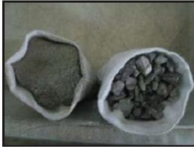
Figure 2.25. Geocontainers with fine crushed concrete and coarse crushed concrete ( Akib et al., 2012 ).
