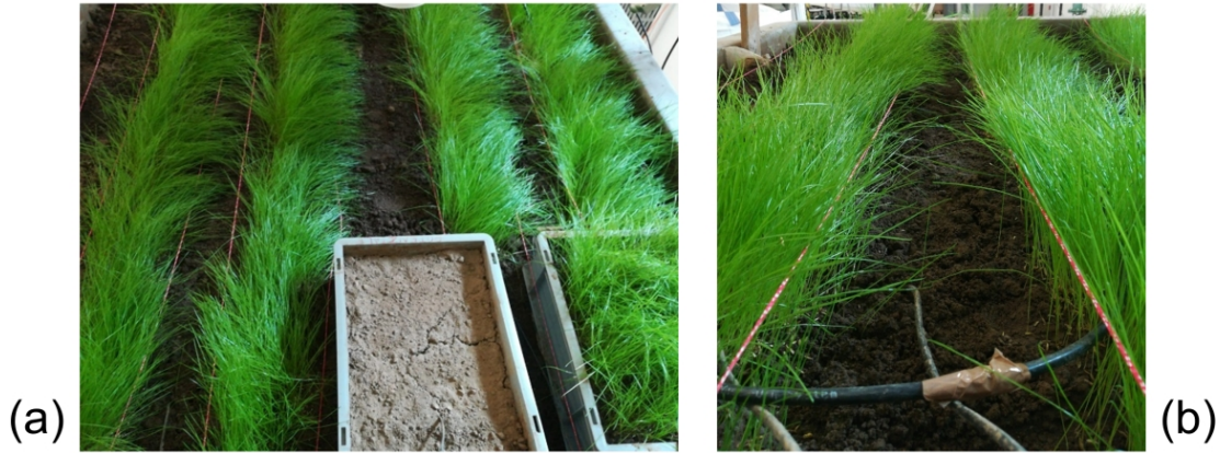
Figure 7.4: Lysimeter view from above after full grass growth (a) and focus on the tape used to avoid irrigation of bare-soil areas (b).
