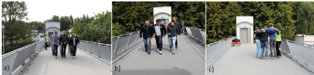
Figure 2.15: Dynamic tests a) walk b) run c) jump [5]
