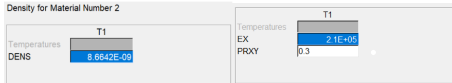
Figure 3.12: Steel material model
