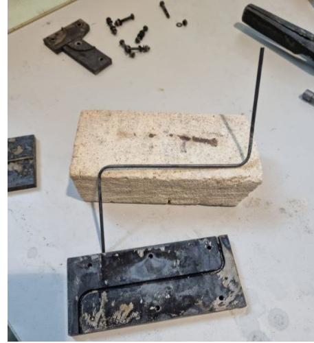
Figure 2: Final outcome of tube shaping
