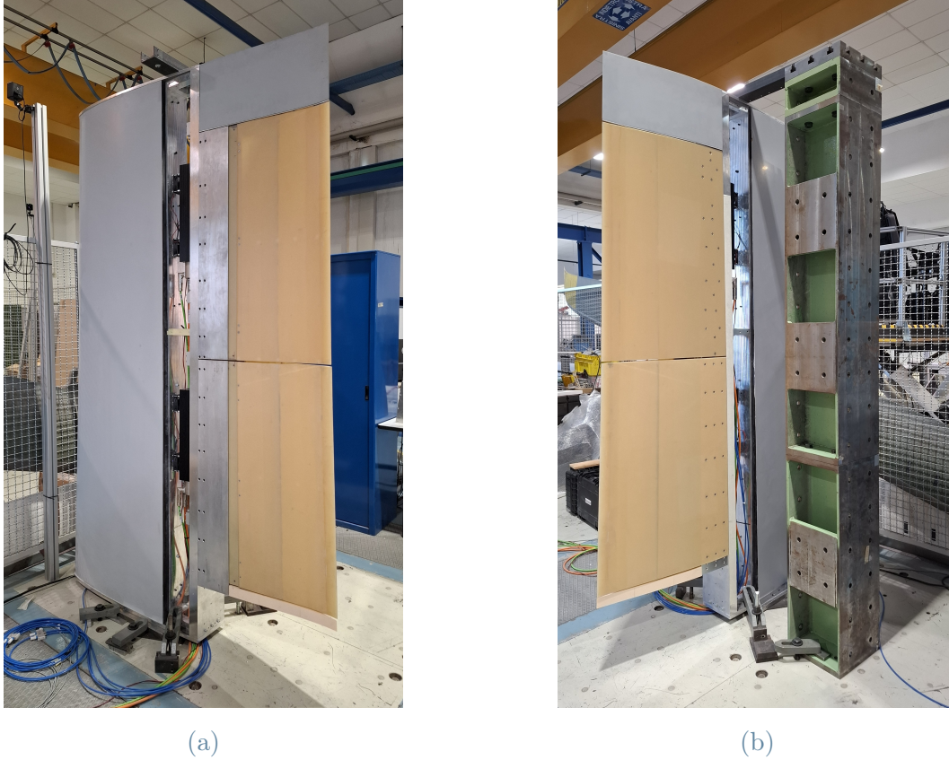
Figure 4.1: Physical prototype of the morphing aileron demonstrator, showing (a) the pressure side and (b) the suction side.
