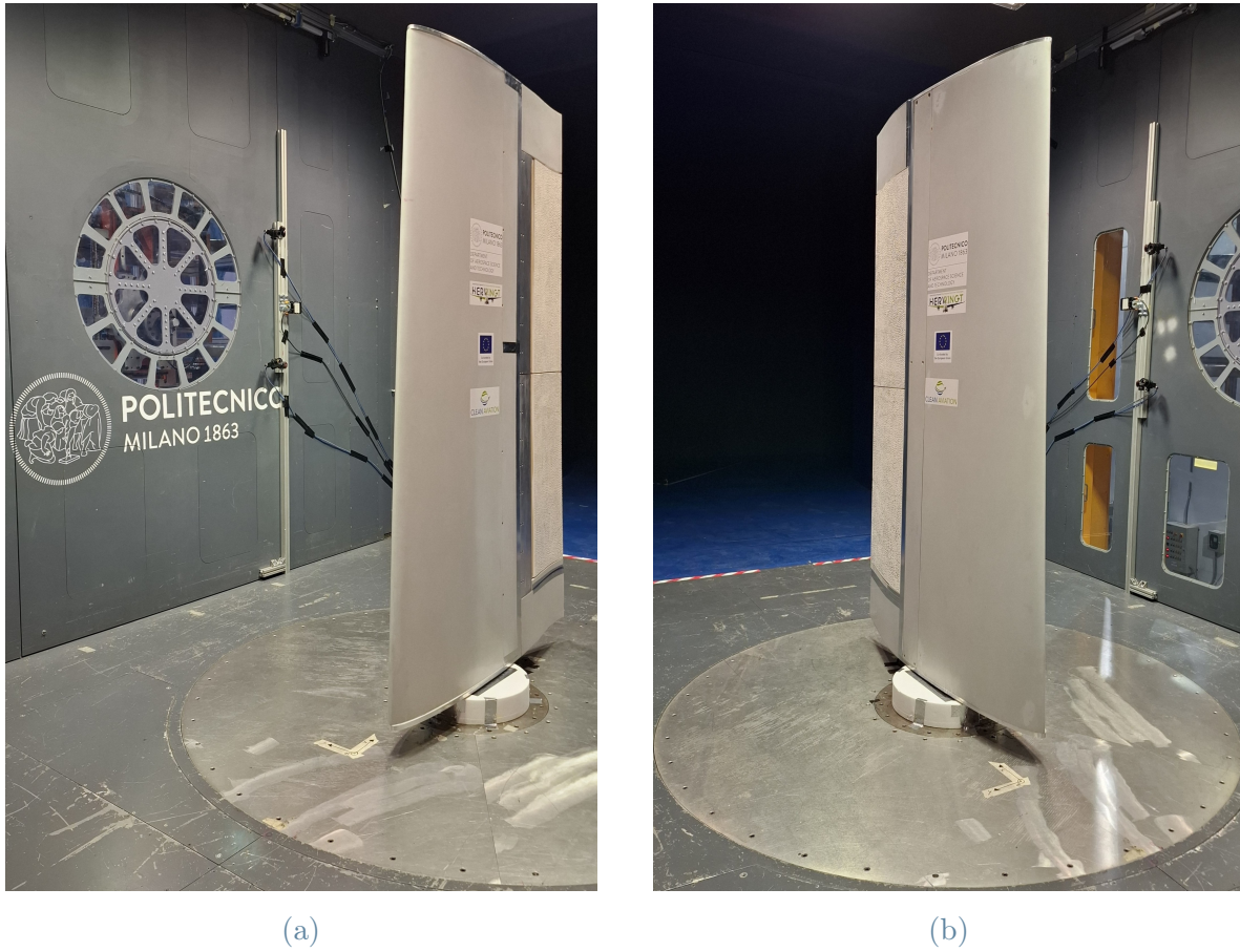
Figure 8.2: Wind tunnel experimental setup: (a) pressure side view; (b) suction side view.
