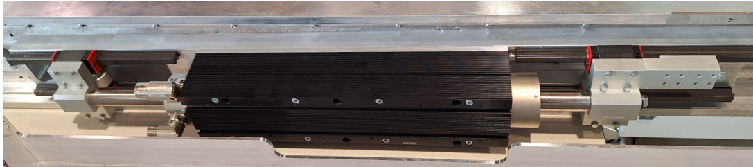
Figure 4.6: Installation details of the linear actuator, viewed from inside the wing-box, highlighting the linear sliding guides on the motor side.
