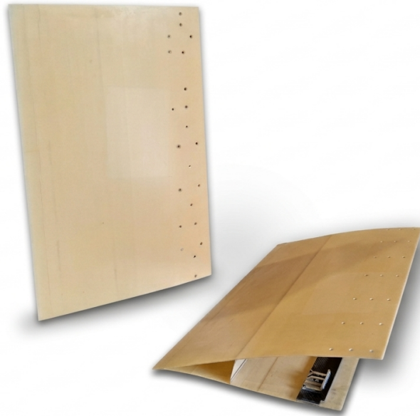
Figure 4.2: The two unassembled segments of the S-glass fibre morphing ailerons.
