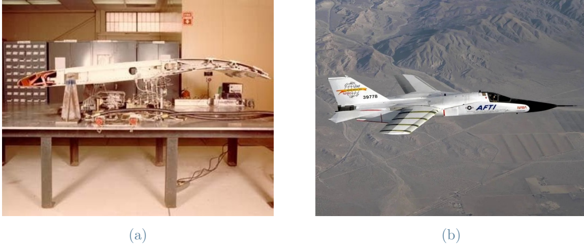
Figure 2.1: (a) shows the MAW airfoil cross-section in its deformed, cambered configuration [41]; (b) shows a modified General Dynamics AFTI/F-111A Aardvark aircraft equipped with MAW during flight [30].
