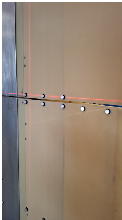
Figure 6.2: Alignment of the reflective markers using a laser level to accurately track the chordwise sections.
