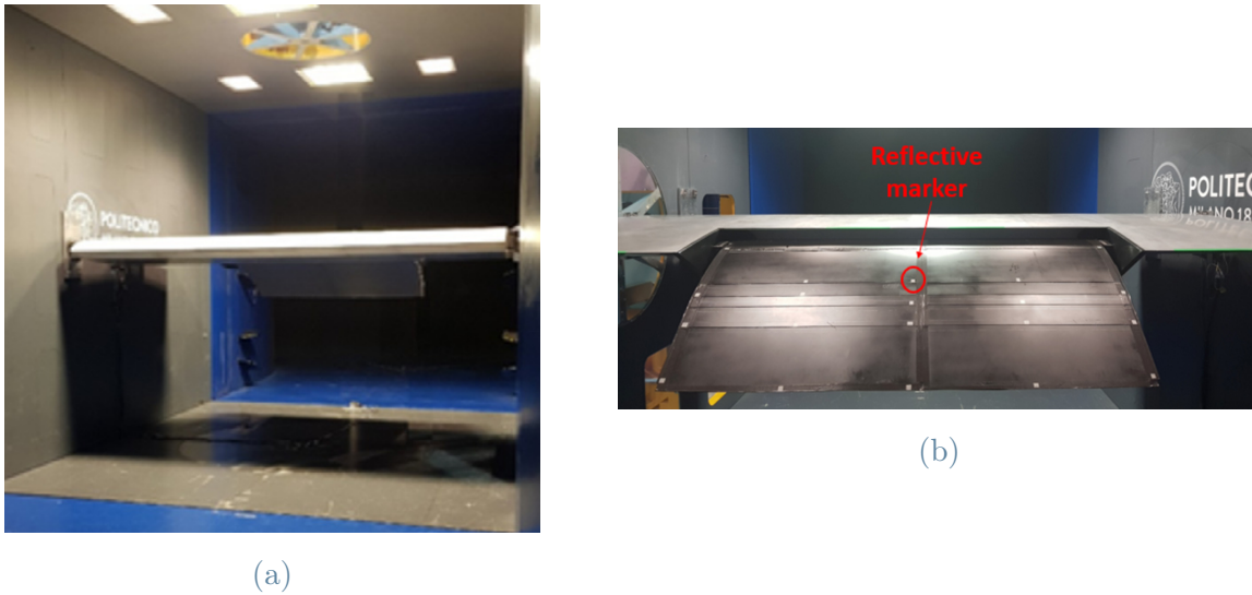
Figure 2.7: (a) shows the SMS model in GVPM facility; (b) shows a close-up of the reflective markers for shape acquisition [5].
