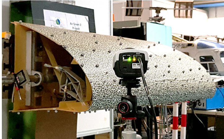
Figure 2.6: Experimental setup of the full-scale morphing droop nose developed by Politecnico di Milano, highlighting the reflective markers used for the Qualisys® tracking [16].
