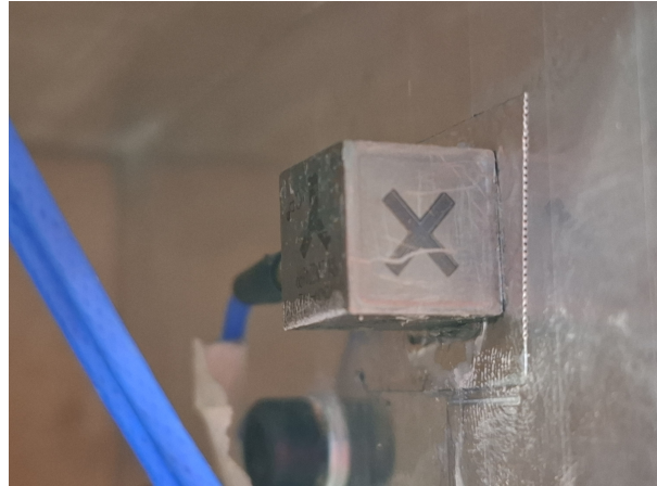
Figure 8.5: A PCB Piezotronics 356A22 triaxial accelerometer mounted on the main spar of the wing-box.
