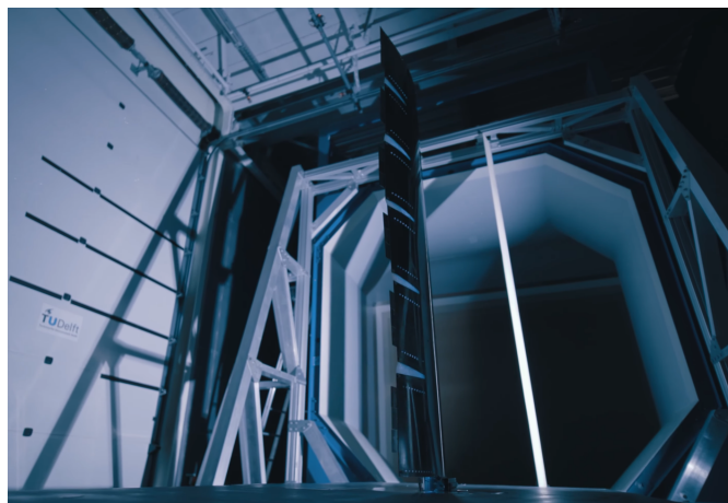
Figure 2.5: The SmartX-Alpha physical demonstrator mounted in the open jet wind tunnel at TU Delft [32].
