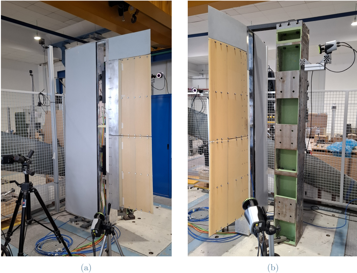
Figure 6.1: Experimental setup for the ground tests using the Qualisys® motion capture acquisition system. (a) and (b) illustrate different views of the arrangement.
