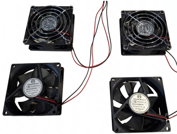
Figure 4.5: The four cooling fans, equipped with protective safety grids, shown prior to installation.
