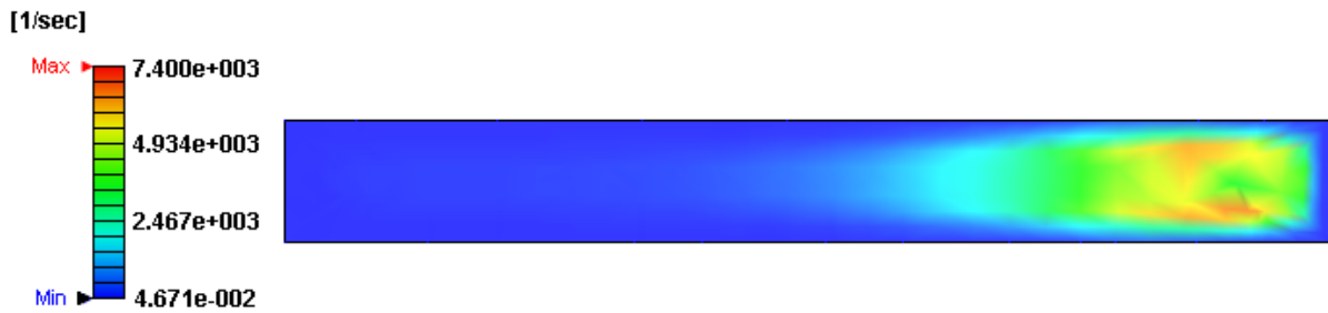
Figure 30. Shear rate at the end of filling across the injection zone cross-section of the GR/50 hv sample of 1.47 mm thickness.
