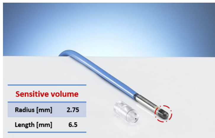
Figure 4.2: Semiflex chamber type 31010 used for the dosimetry calculations. The dimensions of the sensitive volume are reported. Adapted from [79].
