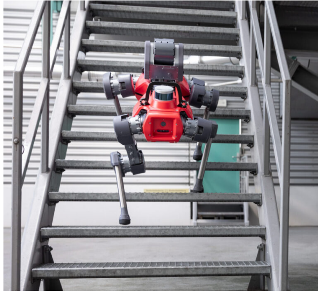
Figure 2.1: Floating base quadrupedal robot, ANYmal, climbing stairs. Source: ANYbotics.
