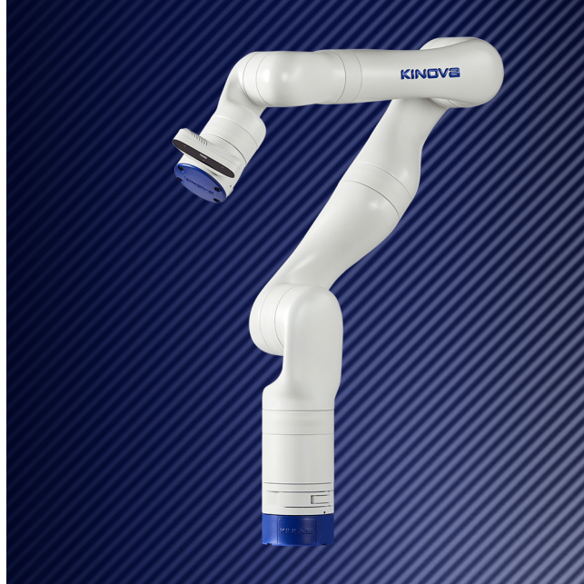
Figure 2.2: Kinova Gen3 7DOF with the vision module attached to the end-effector as provided by Kinova Robotics.
