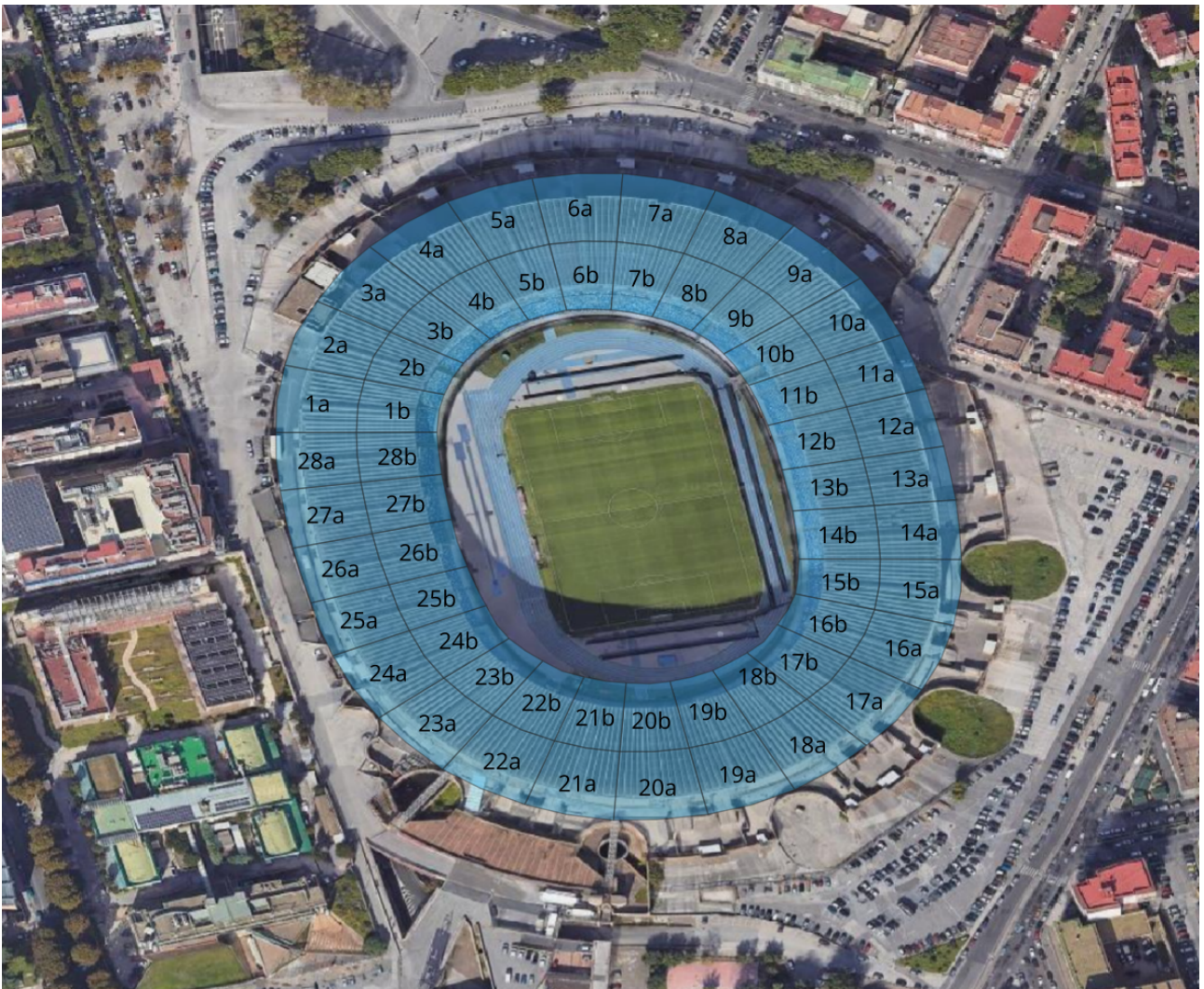
Figure 4.4: Subdivision of the Roof in 28 zones extending towards the city (a) and towards the pitch (b).
