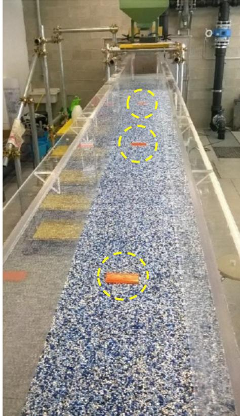
Figure 3.15. Positions of the three metallic plates along the channel (Zucchi 2018).
