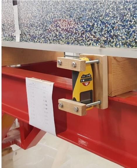
Figure 2.3. Laser distance meter fixed to the channel.
