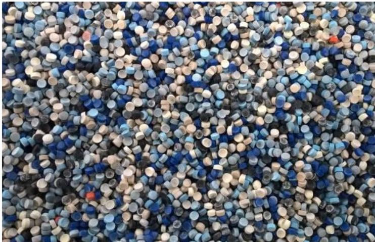
Figure 2.8. PVC grains are used as sediment particles.
