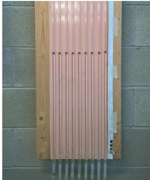
Figure 2.36. Piezometers pipes.
