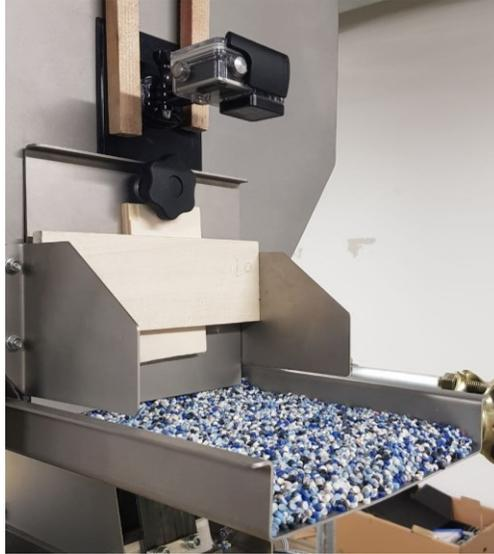
Figure 2.10. Camera positioned above the vibrating channel.
