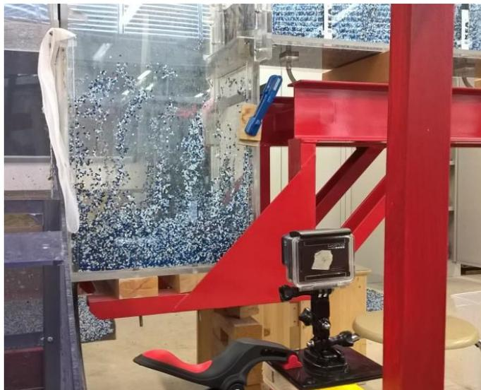
Figure 2.6. Monitored collector located at the downstream of the channel.
