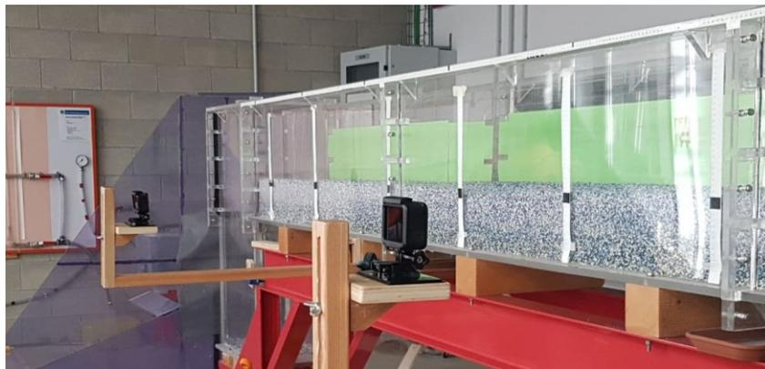
Figure 2.23. Cameras positioned in front of the channel.
