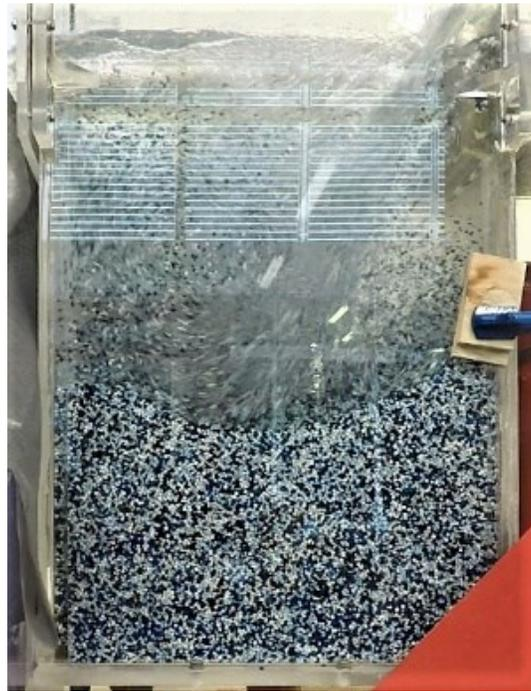
Figure 3.5. Turbulent flow inside the monitored collector.
