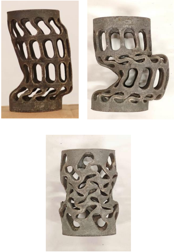
Figure 4.5 Deformed structures at failure
