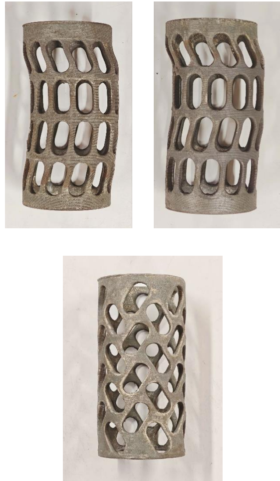
Figure 4.4 Deformed structures under 5mm compression displacement.
