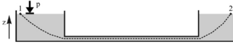
Figure 14. Pipeline connecting two reservoirs considered in equations to calculate the pipe diameter for a desired flow rate.
