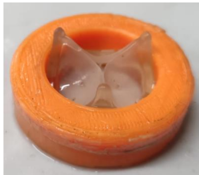
Figure 4.11: Polymeric valve used for tests
