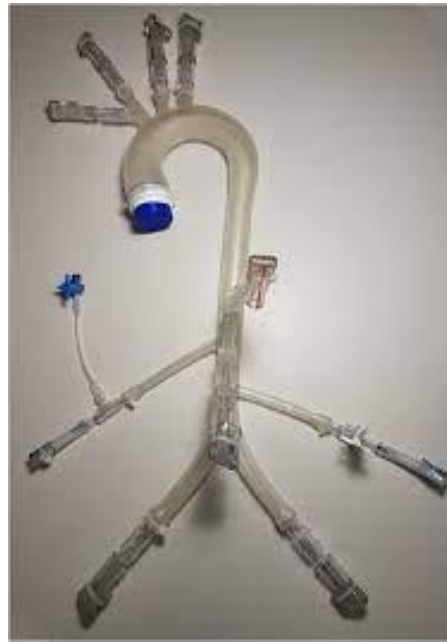
Figure 2.6: Compliant silicone aortic model
