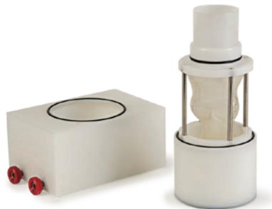
Figure 2.1.2: Compliant aortic conduit
