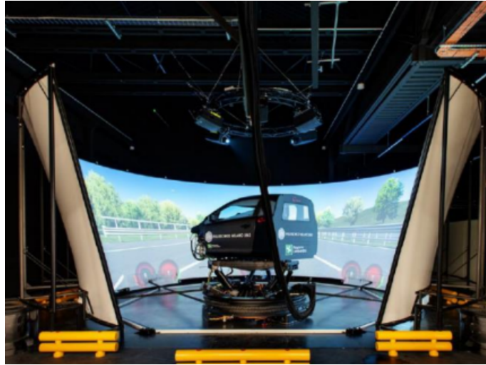
Figure 3.1: Dynamic driving simulator used to perform the simulations.
