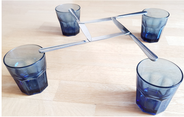
Figure 1.1: Simple example of reciprocal frame
