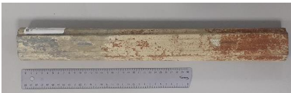
Figure 32 - Visual assessment of corrosion and rust distribution on a vineyard post specimen [34]
